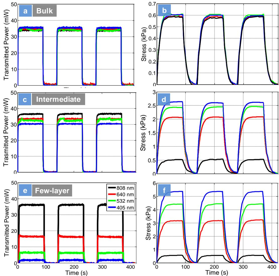
Power transmitted through the sample and the corresponding photomechanical actuation of nanocomposites at different wavelength of light respectively: (a-b) bulk consisting of 100-500 layers; (c-d) intermediate consisting of 10-30 layers and (e-f) few layers consisting of 1-6 layers. The samples were all 0.1 wt. % nanocomposites using LBL process. No pre-strains were applied for these experiments.
