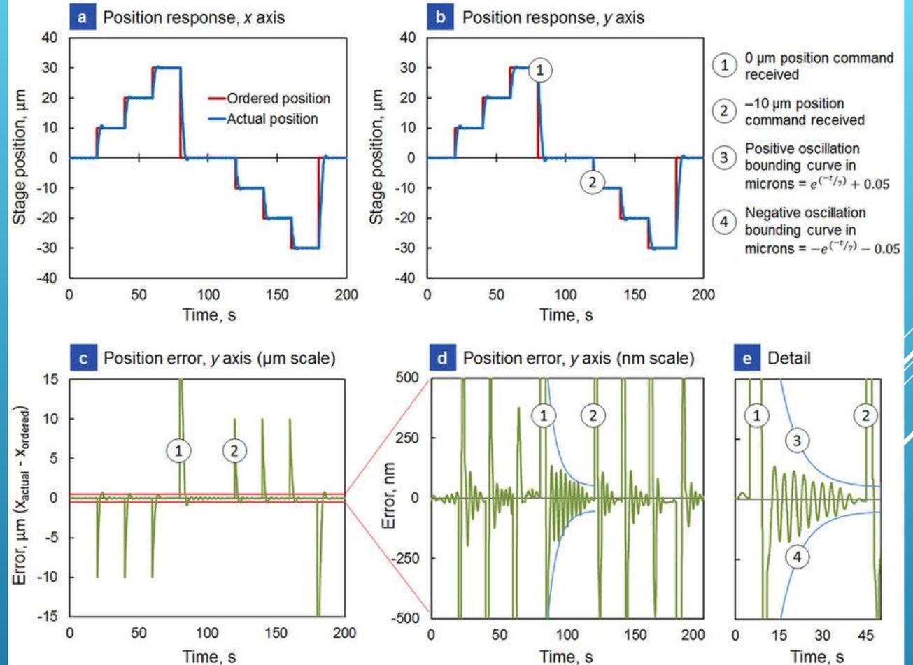
Positioning accuracy:  $\sim 120$  nm.
